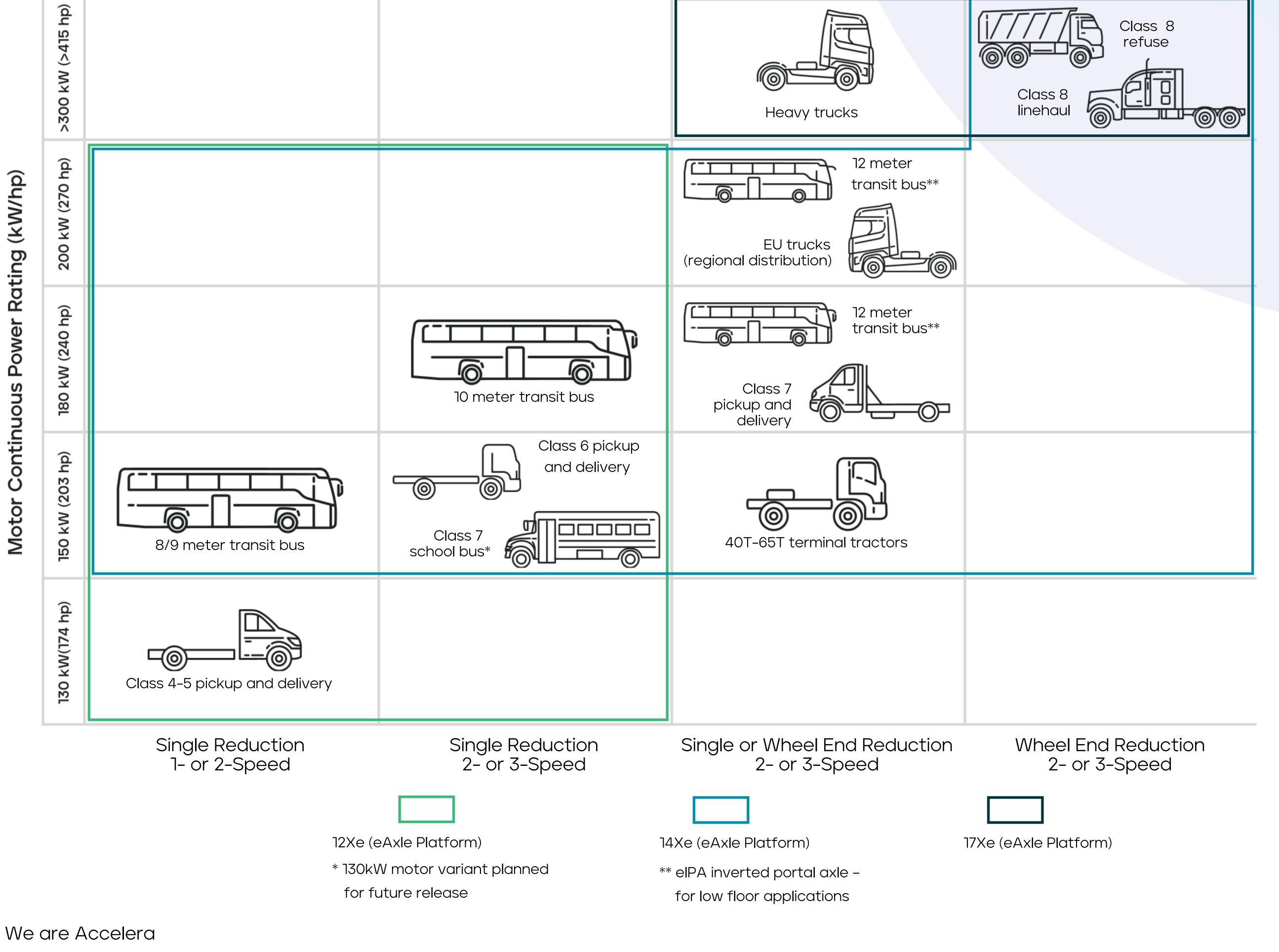
Motor Continuous Power Rating (kW/hp)
